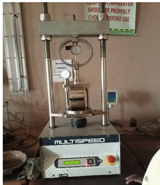
Figure 2: Marshall stability test set-up
