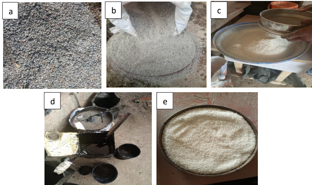
Figure 1: Materials: a. Coarse aggregate b. Fine aggregate c. Mineral filler d. Bitumen e. Sasobit
